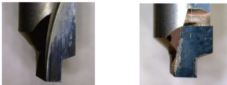
(a) WC end mill without chip breaker (b) PCD end mill with chip breaker
