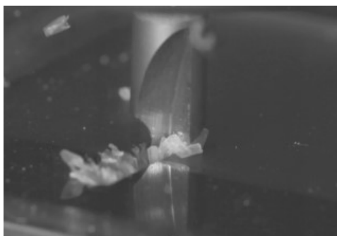
Fig.4-3 Cutting situation clogged with chips.
